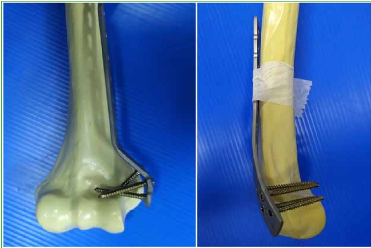
Figure 2. Plastic bone demonstration of poor anatomical reproduction and insufficient joint fixation of a given implant.
