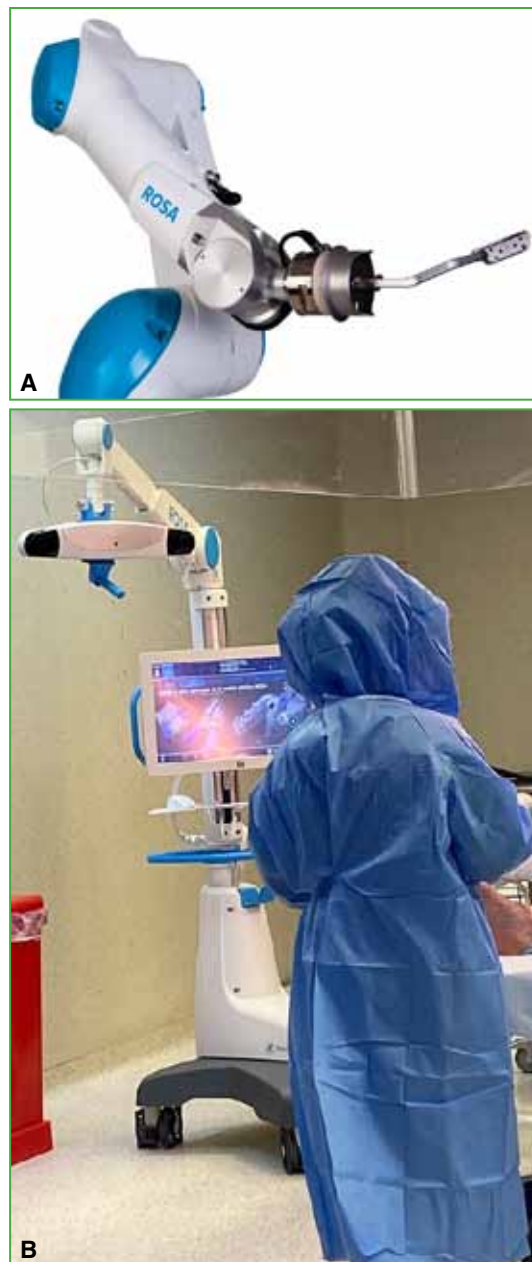
Figura 3. Robotic arm with cutting guide (A) and optics (B).
