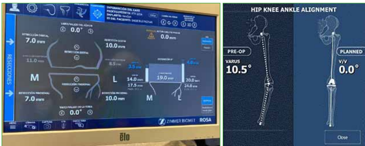
Figure 5. The orientation of the bone resections and the position and size of the implants allow adjustment of the gaps in extension and flexion, and the final alignment of the entire limb. Modifying all of these values will give instant feedback on alignment and gaps.
